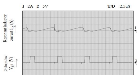
Fig.11. Resonant inductor current ( i_{Lr} ) and auxiliary switch pulse ( V_{g2} ).
