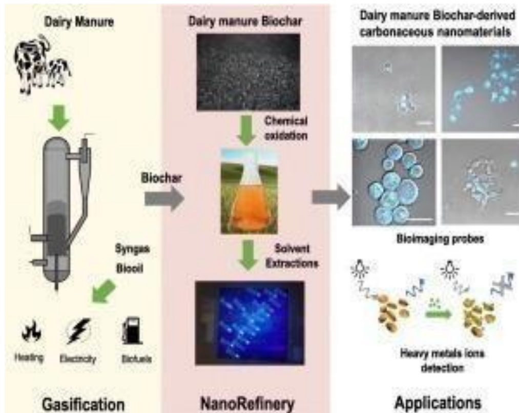
Figure:2.Potential option is the use of carbonaceous nanomaterials due to their specific properties that make them suitable to be used as technological sensors
