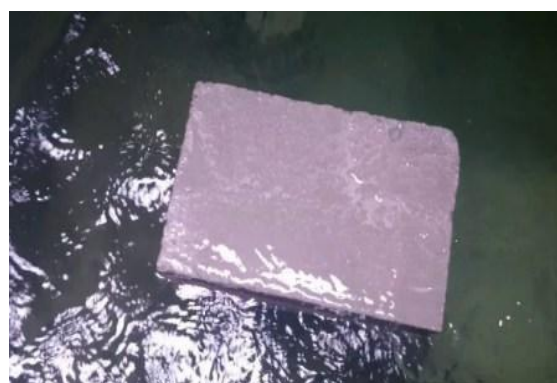
Fig 2 Shows Light Weight Floating Brick Floating in water
