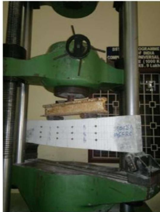
Flexural test on beam with BGC3 mix
