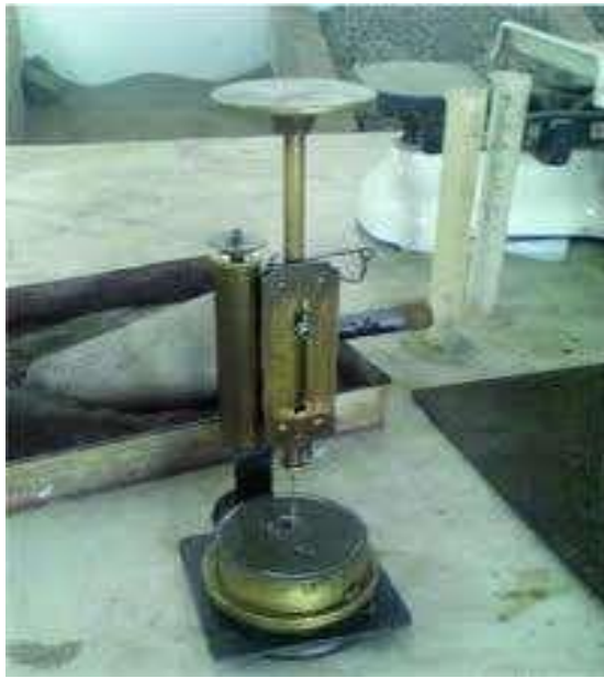
Fig5.2 Vicat Apparatus to find initial setting time
