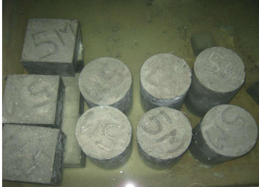
Fig 7.8 Specimen in Curing Tank for Curing
