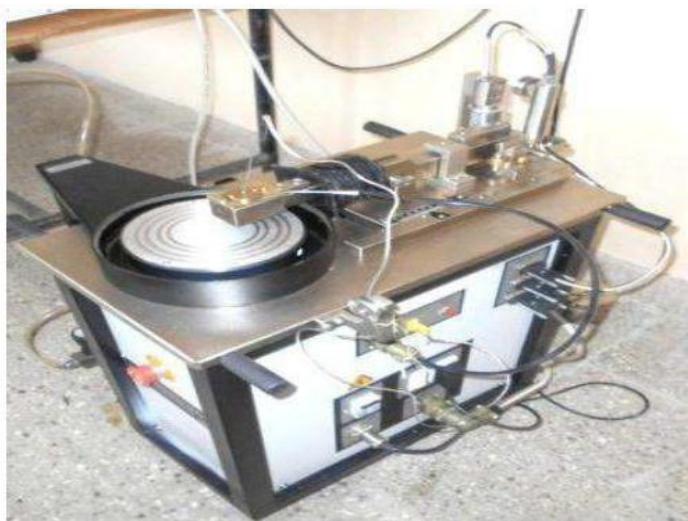
Fig.2: Pin on Disc test setup
